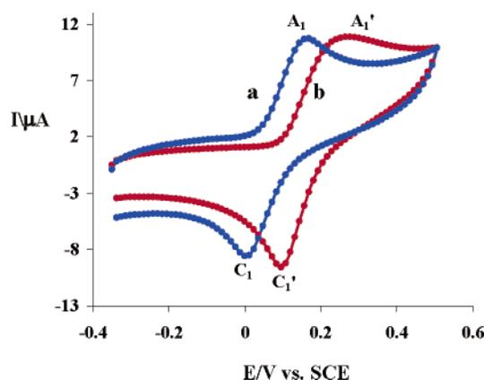
**FIGURE 3.** Cyclic voltammogram of (a) 1 mM 4-*tert*-butylcatechol (**1c**), (b) 1 mM obtained product (**4c**) at glassy carbon electrode in water/acetonitrile (50/50) solution containing 0.2 M phosphate buffer (pH = 7.2). Scan rate: 50  $\text{mV s}^{-1}$ ;  $t = 25 \pm 1^\circ\text{C}$ .
