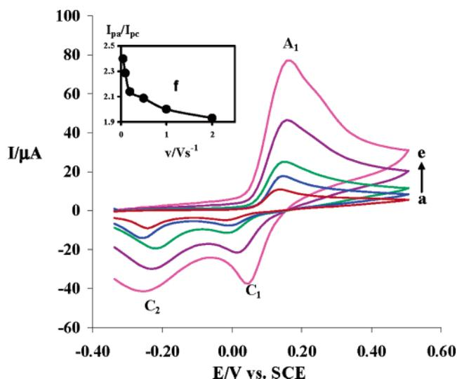
**FIGURE 2.** Typical cyclic voltammograms of 1 mM 4-*tert*-butylcatechol (**1c**) in the presence of 1 mM 2-mercaptobenzoxazole (**3**) at a glassy carbon electrode in water/acetonitrile (80/20) solution containing 0.2 M phosphate buffer (pH = 7.2) Scan rates from (a) to (e) are: 50, 100, 200, 500, and 1000  $\text{mV s}^{-1}$ , respectively. (f) Variation of peak current ratio ( $I_p^{A_1}/I_p^{C_1}$ ) versus scan rate;  $t = 25 \pm 1^\circ\text{C}$
