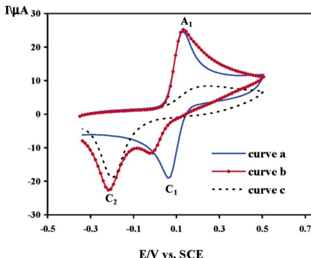
**FIGURE 1.** Cyclic voltammograms of 1 mM 4-*tert*-butylcatechol (**1c**). (a) In the absence and (b) in the presence of 1 mM 2-mercaptobenzoxazole (**3**), (c) 1 mM 2-mercaptobenzoxazole (**3**) in the absence of 4-*tert*-butylcatechol (**1c**) at glassy carbon electrode in water/acetonitrile (80/20) solution containing 0.2 M phosphate buffer (pH = 7.2). Scan rate: 200 mV s<sup>-1</sup>; *t* = 25 ± 1 °C.
